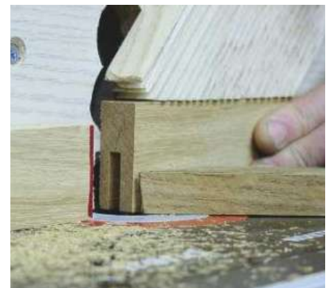
▲ Pic.3 Routing grooves in the rails for the side panels
